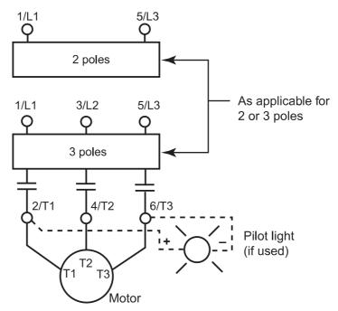
**NOTE:** The lamp is polarity sensitive in DC applications.
